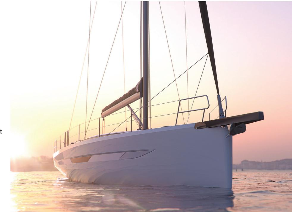
**Above:** active aft-quarter chines come into play when the E6 heels over, boosting the form stability of the hull. The waterline beam is relatively narrow to ensure good performance in light airs. **Right:** The cruising setup includes a big bathing platform and stern boxes with a BBQ grill and fridge inside – great for enjoyment at anchor, removable for racing
