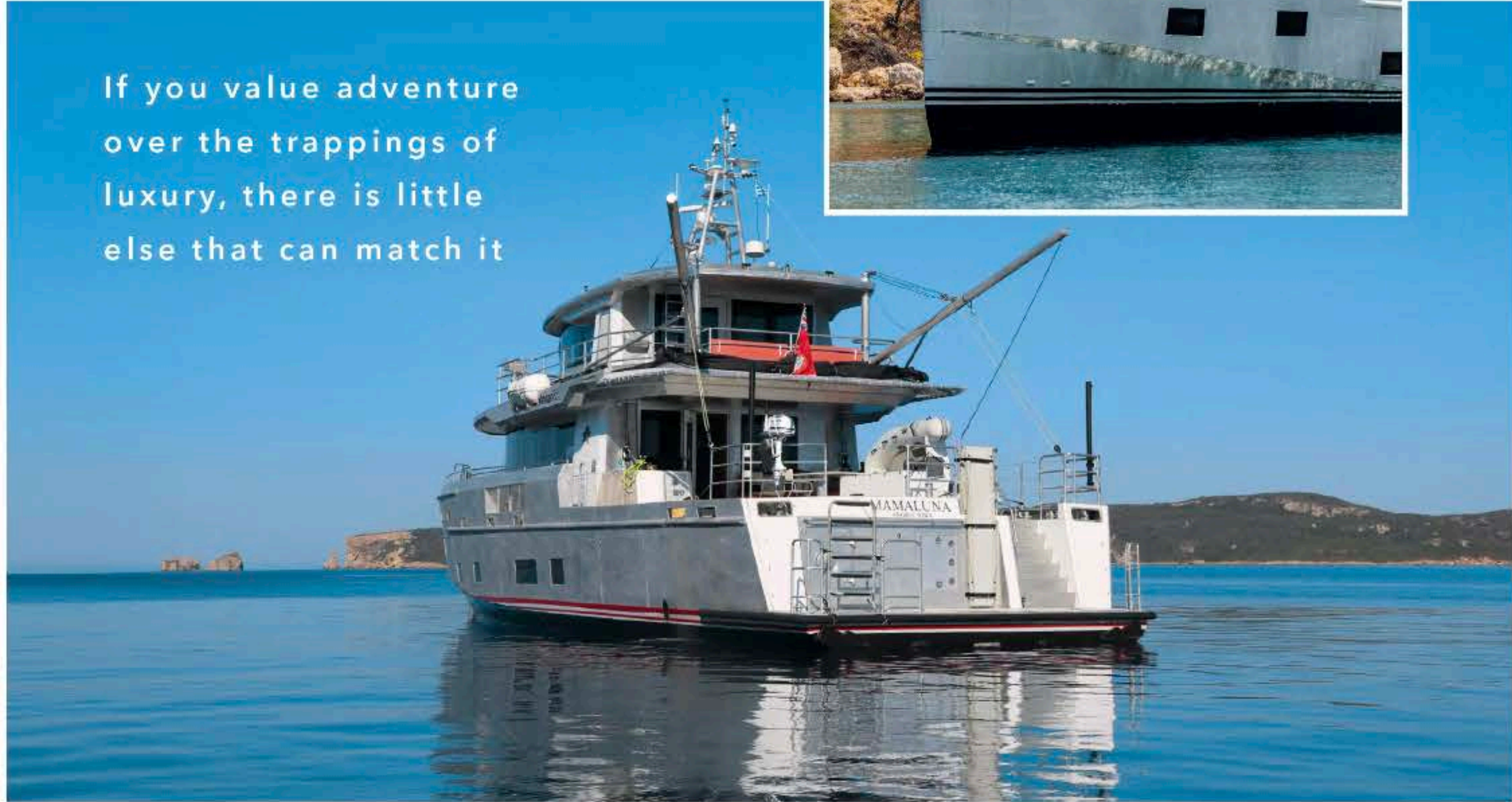
BELOW: Twin outriggers double as tender lifts but also act as passive stabilisers when fitted with flopper stoppers at anchor
